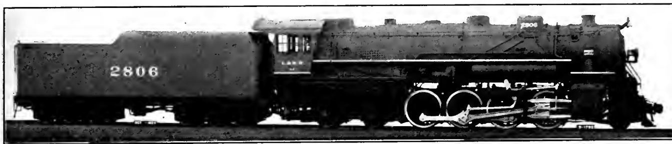
2-8-4 Type Locomotive of the Chicago & North Western Railway—Built by the American Locomotive Company
